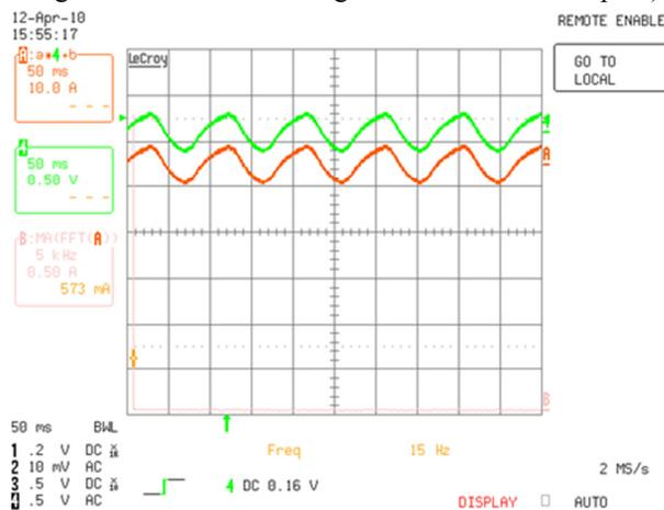
Figure 4: output current oscillation (DC set is 100 A), on a 30 V – 110 A COTS PS, before adjusting the regulation.
