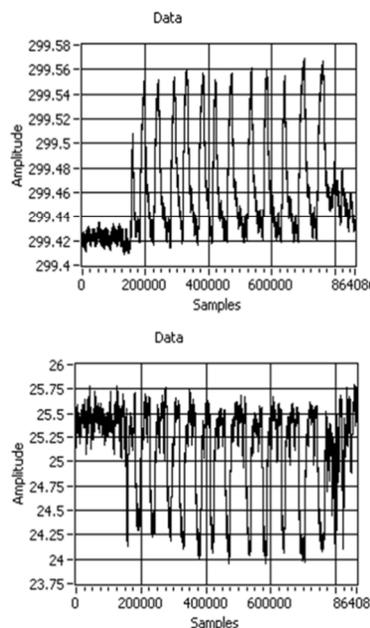
Figure 3: effect of room temperature on the stability test of PS over 24 hours (Top output current [A], bottom room temperature [°C]).
