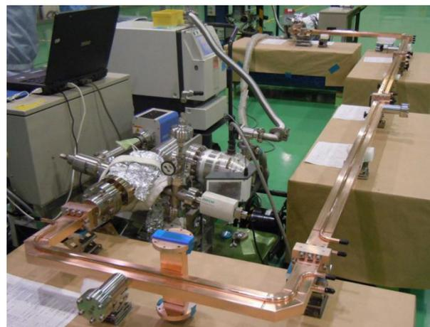
Figure 4: Vacuum test of vertical waveguide at MHI factory.
