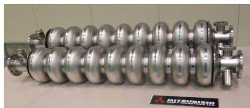
Figure 6: TESLA-shape cavities.
