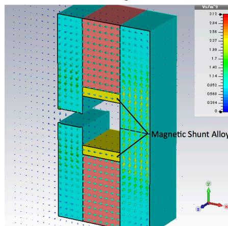
Figure 6: Magnetic field distribution in a prototype LGB with a magnetic shunt.
