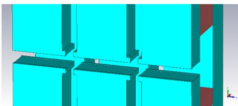
Figure 4: Nose structure for compensation of field dip between LGB poles.
