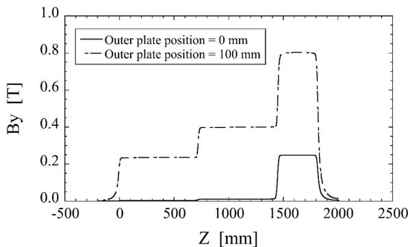
Figure 3: Simulated longitudinal field distributions for outer plate position at 0mm and 100mm.
