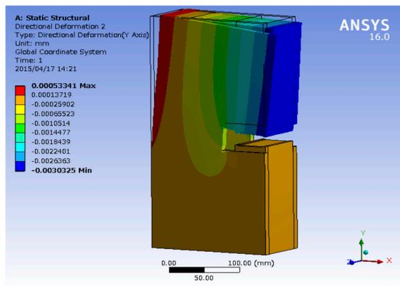
Figure 8: Deformation of a prototype LGB.
