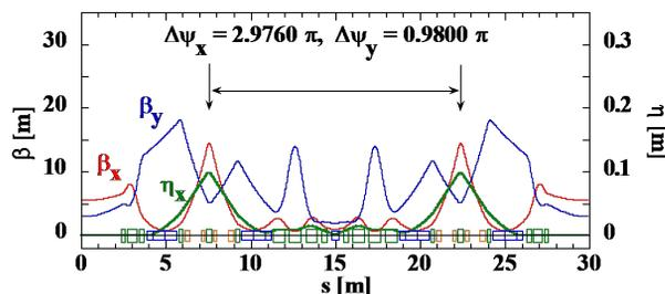
Figure 1: A unit cell of the 5-bend achromat optics for SPring-8-II.
