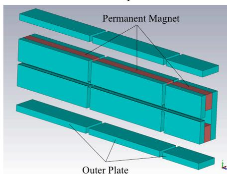
Figure 2: Longitudinal gradient bend with outer plates.
