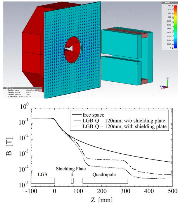
Figure 9: Magnetic field distribution in a shielding plate (above) and that on a beam axis (below).
