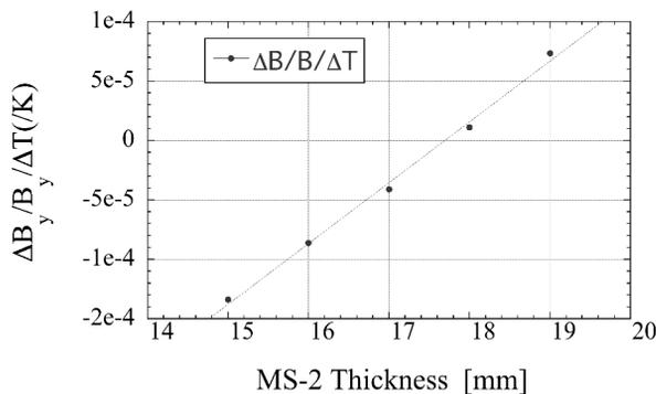
Figure 7: Simulated optimization for the thickness of a magnetic shunt material for the prototype LGB.
