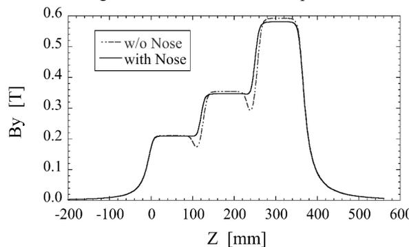
Figure 5: Compensation of field dip between LGB poles using nose structures.
