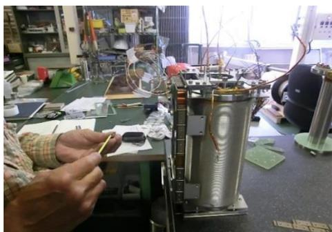
Figure 6: Steering coil assembly on the main solenoid.
