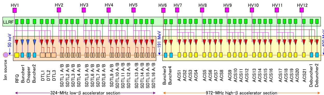
Figure 1: Outline of RF systems and RF cavities of the upgraded J-PARC 400-MeV linac.
