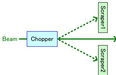
Figure 7: Schematic diagram of one chopper with two scrapers at the J-PARC linac.
