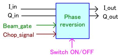
Figure 8: Phase-reversion function block inserted in the FPGA output circuits.
