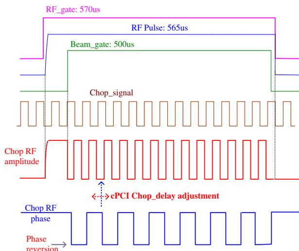
Figure 9: Schematic view of timing signals for the chopper station and output RF amplitude and phase for the chopper cavity.
