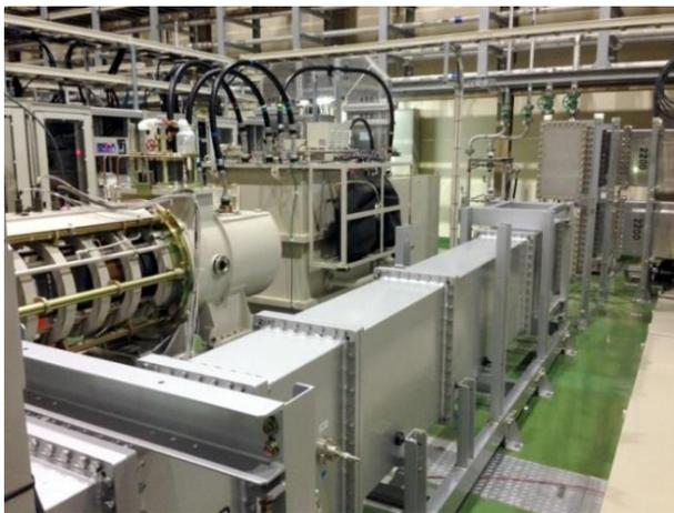
Figure 2: Waveguide system for the upgraded RFQ with one input port.
