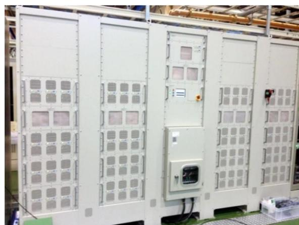
Figure 6: R&K 120 kW amplifier for the chopper cavity.
