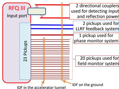
Figure 3: Directional couplers and signal pickups for the upgraded RFQ RF system.
