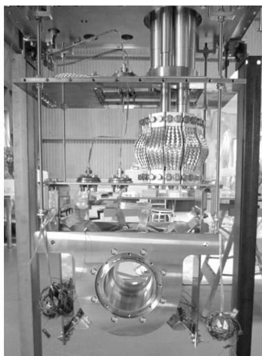
Figure 4: Coils hung from the top flange.
