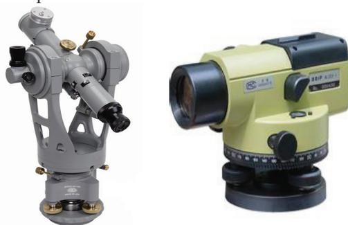
Figure 4: The Theodolite and Level.
