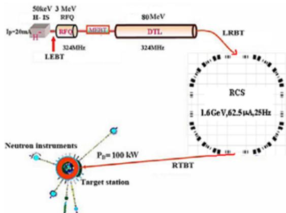
Figure 1: The structure diagram of CSNS.
