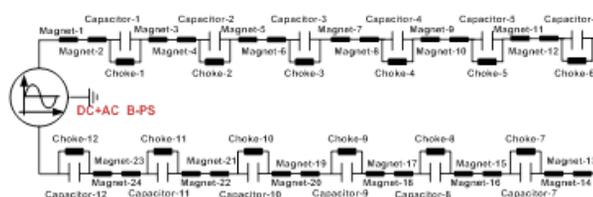
Figure 3: Resonant network of the RCS Dipole PS.
