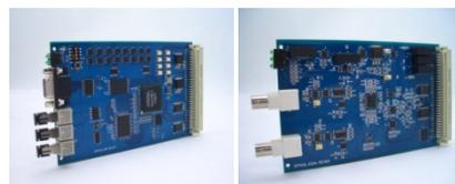
Figure 2: The DPSCM for CSNS Power Supply.
