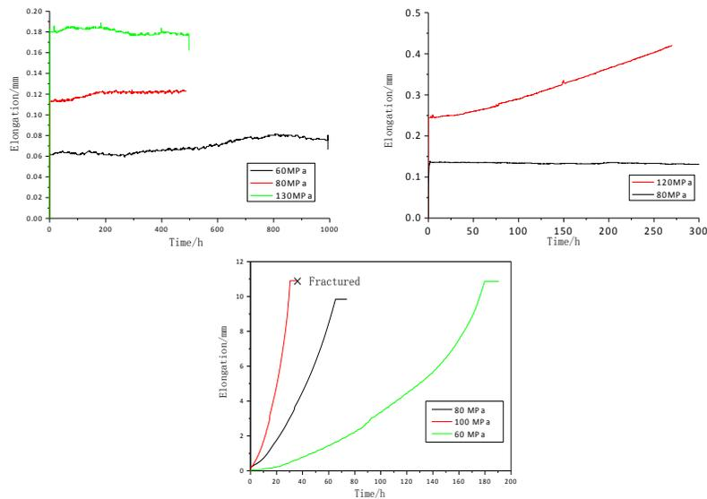
Figure 5: Creep curves (L: at 100 °C; M: at 150 °C; R: at 200 °C).
