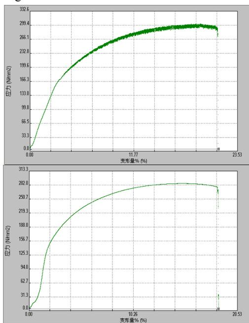
Figure 2: Tensile curve (U: at 25 °C; D: at 100 °C).
