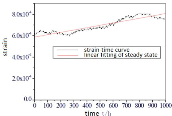
Figure 6: Linear fitting for creep curve at 100 °C and 60 MPa.
