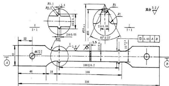
Figure 4: Sample dimensions for creep experiment.
