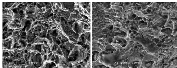
Figure 3: Scanning at fracture cross sections (U: at 25 °C; D: at 100 °C).
