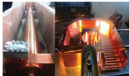
Figure 4: Prototype of the J-type accelerating tube.
