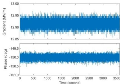
Figure 4: Long-term running of LLRF control system.
