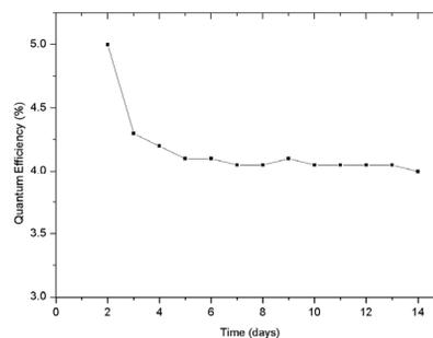
Figure 3: QE of Cs<sub>2</sub>Te cathode.
