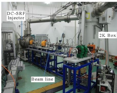
Figure 2: Beam line of the 3.5-cell DC-SRF injector.
