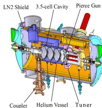
Figure 1: Schematic view of the DC-SRF photoinjector.
