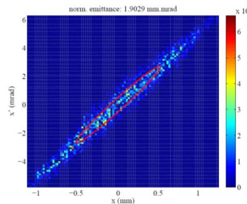
Figure 6: Measured emittance of electron beam.
