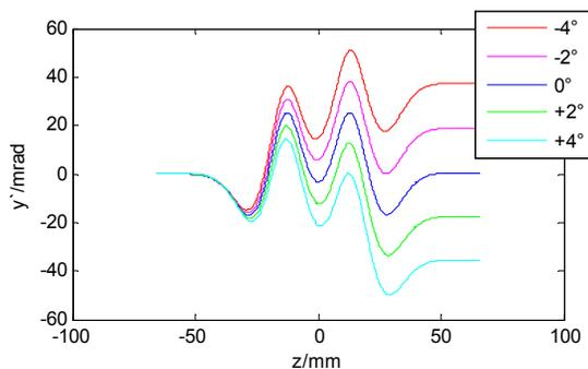
Figure 6: Vertical deflection along z axis with different phases.
