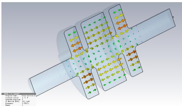
Figure 2:  $\pi$ -mode needed in the RF cavity.
