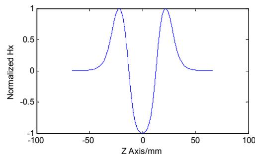
Figure 4: Normalized  $H_x$  along z axis.
