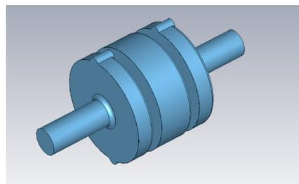
Figure 1: 3D-design of the deflector.
