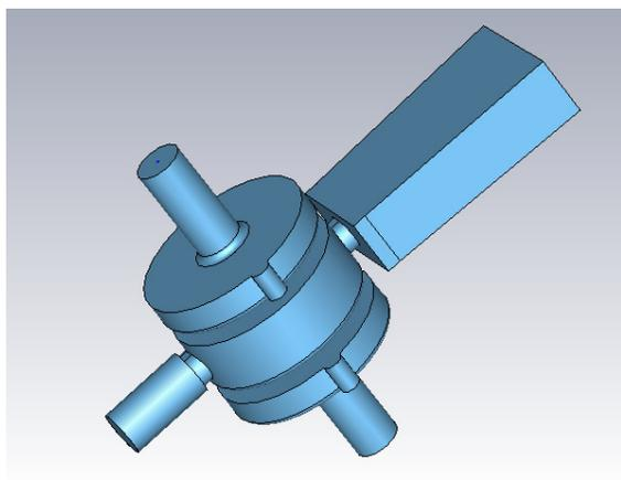
Figure 7: The RF deflector with coupler.
