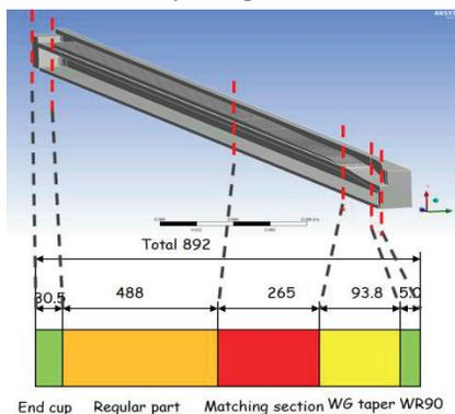
Figure 2: Five functional sections of the load.
