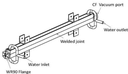
Figure 1: CERN double band SS430 dry RF load.
