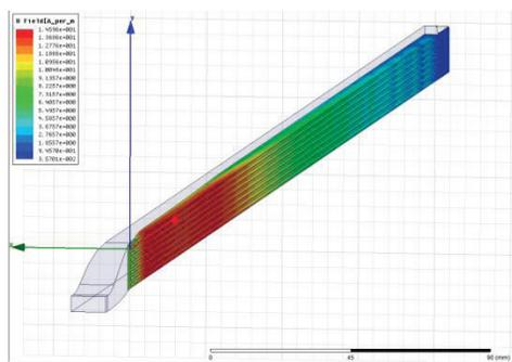
Figure 3: Magnetic field of the load in HFSS.
