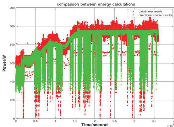
Figure 6: Average power comparison between RF measurements and calorimetric power measurements.
