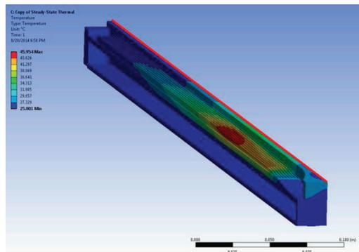
Figure 4: Temperature distribution of the load in ANSYS.
