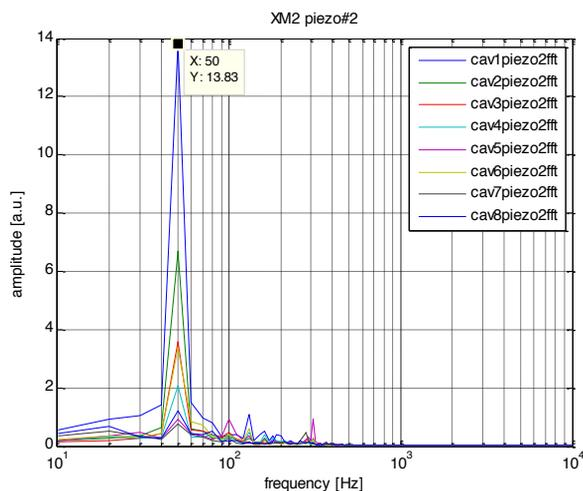
Figure 1: Microphonics measurement at XM-2 module.
