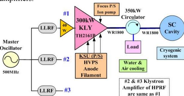
Figure 1: Klystron Amplifier at PLS-II RF system.
