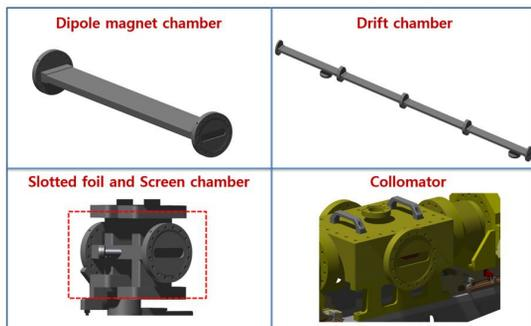
Figure 7: 3D modelling of unified beam chamber.
