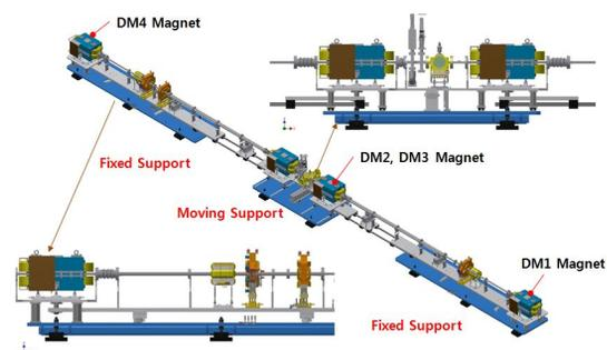
Figure 3: 3D modelling of BC support system.
