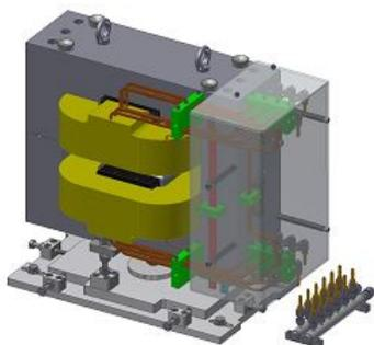
Figure 4: 3D modelling of Dipole Magnet D1.
