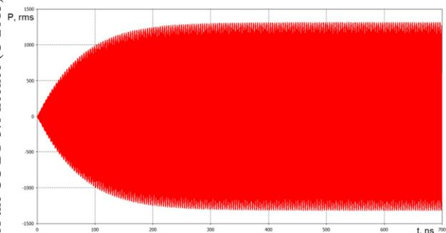
Figure 7: Output signal time dependence in the tuned cavity.
