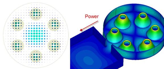
Figure 4:  $TH_{020}$  wave in resonator and the power output waveguide.
