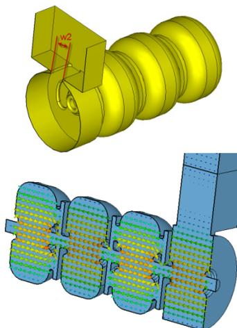
Figure 9: Tuned biperiodic accelerating structure After the connection these two structures together the connecting waveguide length (Fig. 10) was varied till resonant frequency (Fig. 11) stopped to depend from it.
