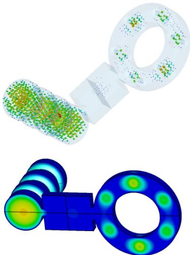
Figure 11: Operating mode obtained in the eigen mode solver.
