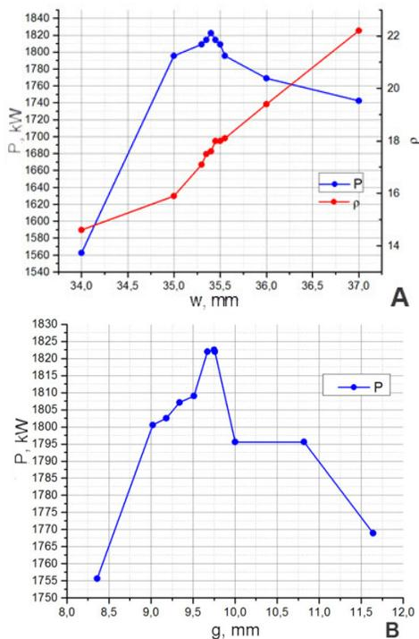
Figure 6: A. Power and VSWR dependence from the window width; B. Power dependence from the gap size.
