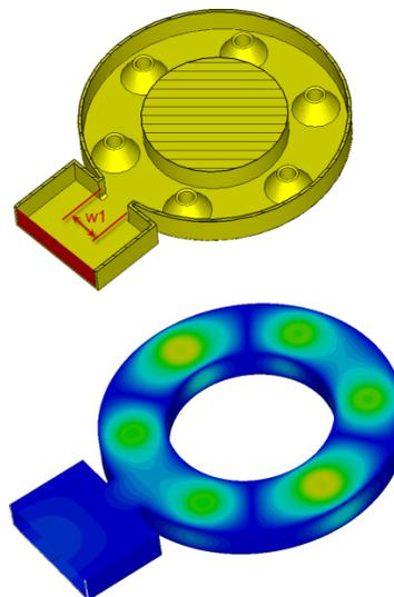
Figure 8: Coaxial IOT geometry and field distribution.
