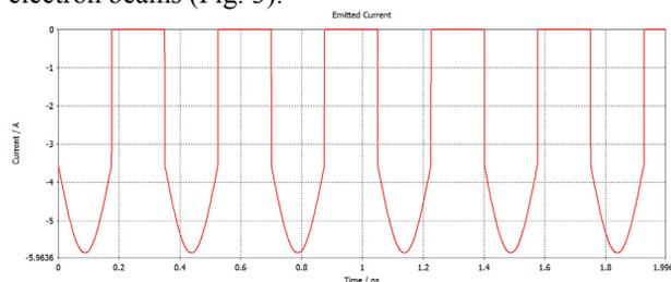
Figure 3: Emitted current from the one cathode.
