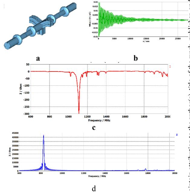
Figure 11: a) Array of 4 cells with ridged waveguide; b) transverse wake potential; c) transverse impedance; d) longitudinal impedance.
