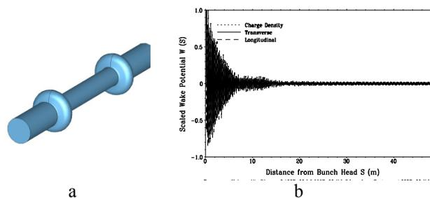
Figure 6: a) Array of 2 cells with grooved beam pipe; b) transverse wake potential.
