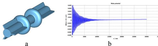
Figure 5: a) Array of 2 cells with fluted beam pipe; b) transverse wake potential.
