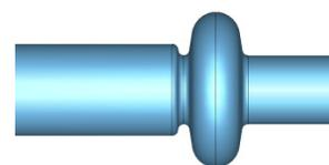
Figure 2: Cavity with grooved beam pipes.
