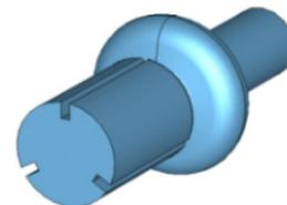
Figure 4: Structure with ridged beam pipe.
