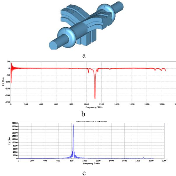
Figure 10: a) array of 2 cells with ridged waveguides; b) transverse impedance; c) longitudinal impedance.
