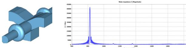
Figure 9: a) Array of 2 cells with attached wide waveguide; b) longitudinal impedance.
