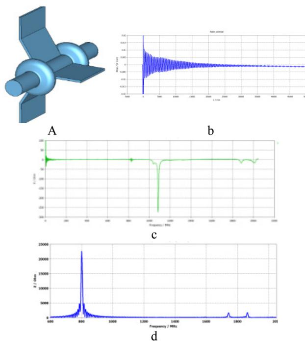
Figure 8: a) Array of 2 cells with attached waveguide; b) transverse wake potential; c) transverse impedance; d) longitudinal impedance.
