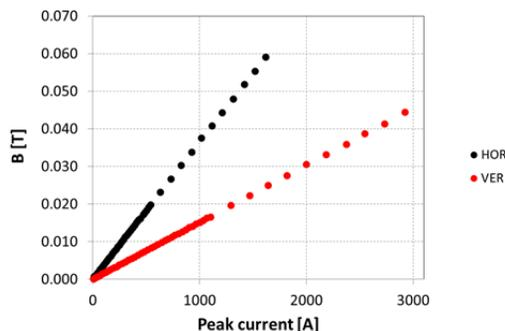
Figure 7: Magnetic field linearity with current pulse.
