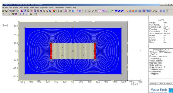
Figure 3: OPERA 2d simulation of the HOR pinger magnet.
