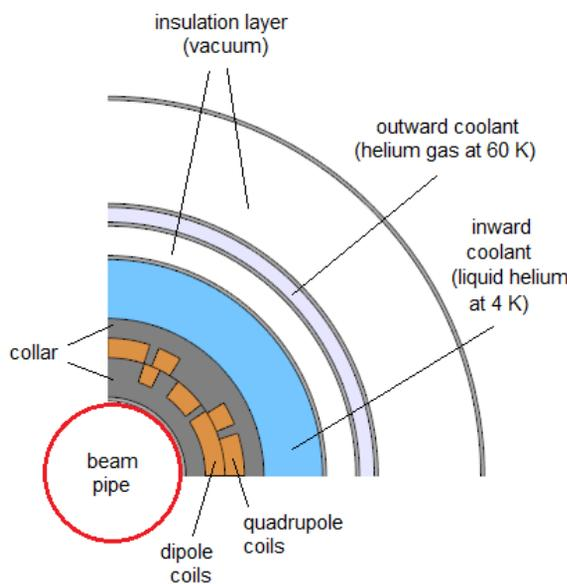
Figure 2: Sketch of the transverse layers to be considered for cryogenic cooling of the gantry.
