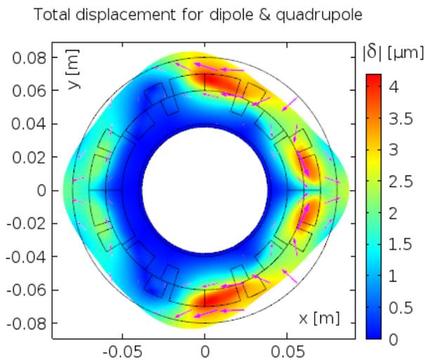
Figure 6: Mechanical deformations due to the combined effects of dipole and quadrupole magnetic fields.
