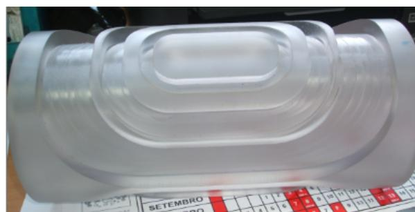
Figure 5: Prototype of a magnet support on which copper-made coil blocks will be wound.
