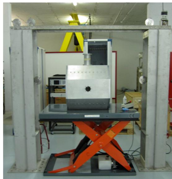
Figure 1: Bead pull system and cold model of RFQ in aluminium.
