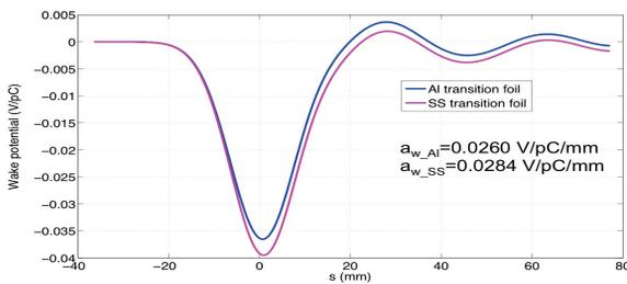
Figure 3: SS and Al transition foil wakepotential comparison.
