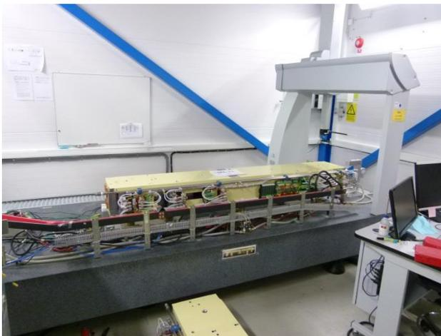
Figure 3: The Hall probe mapping bench.
