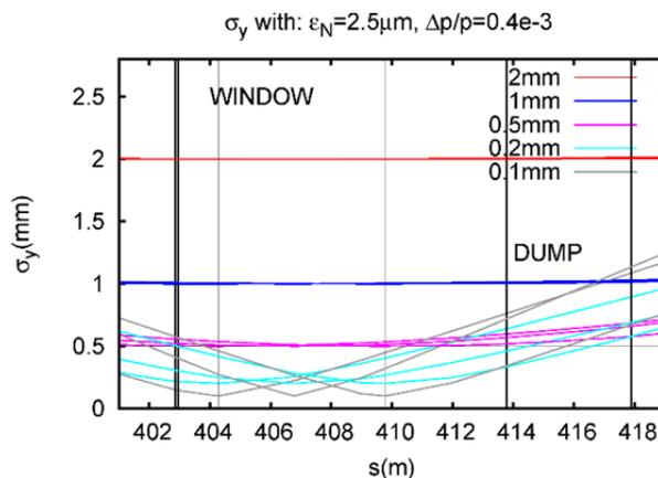
Figure 4: Calculation of the vertical beam size of a proton beam similar to Fig. 3.
