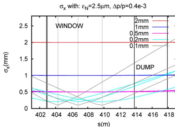
Figure 3: Calculation of the horizontal beam size of a proton beam with nominal emittance as a function of the longitudinal position in the region of the experimental area for different focal point positions and for different focal spot sizes.
