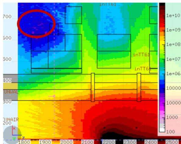
Figure 6: Prompt radiation levels around the target area and the proposed electronics positions in TT61 (red circle). The radiation levels are shown in fluence/cm<sup>2</sup> (hadrons > 20 MeV) and for  $3.7 \times 10^{12}$  protons impinging on a thick target.
