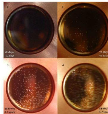
Figure 6: Pictures of the cathode 1) 8.26.2013 (shortly after installation) 2) 9.30.2013 3) 5.14.2014 4) 4.24.2015. An estimated 600 spots developed during RF conditioning. The photocathode QE is 2% after 1.7 years of operation.
