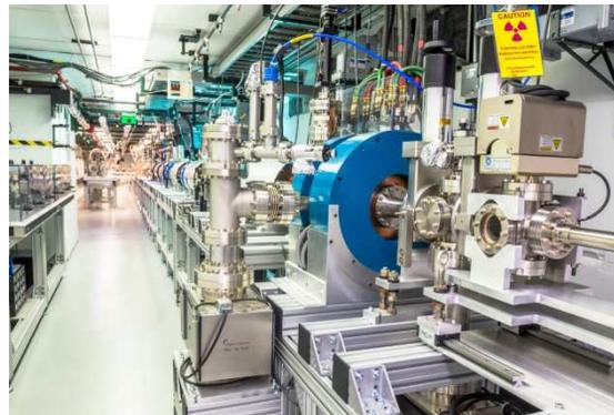
Figure 1: AWA upgrade: The new drive beam photocathode gun, looking in the direction of the beam. In the foreground is the cathode load-lock system.
