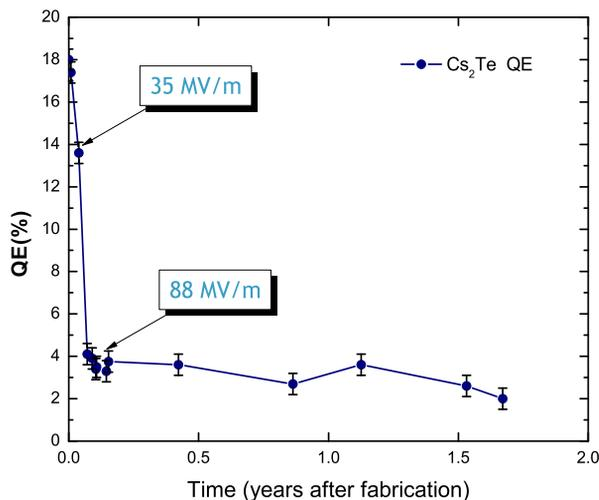
Figure 5: QE vs. time for the AWA drive gun photocathode installed in August 2013 and still operating today. The photocathode QE was initially about 18% in the deposition chamber and is currently about 2%.
