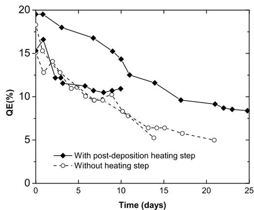
Figure 2: QE vs. time of four Cesium telluride photocathodes. After fabrication, two photocathodes (black diamonds) were heated for 2-3 days at 120° C. The result: the QE decay rate is significantly reduced.
