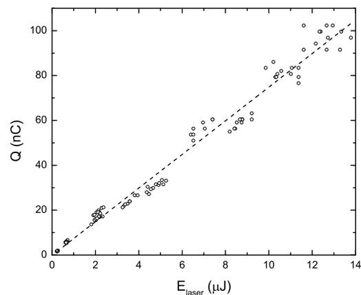
Figure 3: Shot-by-shot charge vs. laser energy data using a 22 mm laser spot on the Cs<sub>2</sub>Te photocathode. The peak RF electric field on the cathode was 84 MV/m. The good linear fit indicates no space-charge effects. From the slope, QE > 3%.
