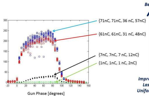
Figure 4: Summary plot of bunch-train generation at AWA (total charge per train). The maximum charge per train is a function of the laser profile quality. Individual charges sum to the total charge, indicating that there is no bunch-position QE dependence for the four bunch train.
