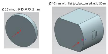
Figure 3: Specimen types: thin discs and slugs.
