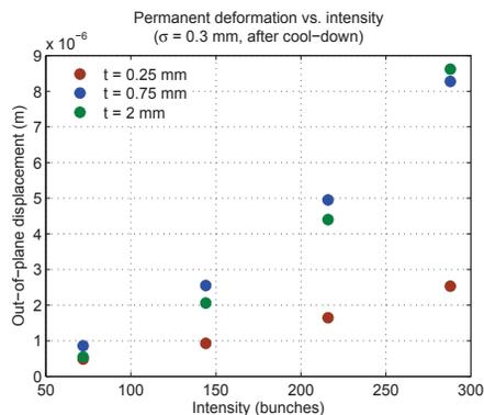
Figure 7: Peak out-of-plane surface deformation after cool-down.
