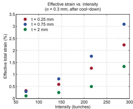
Figure 6: Peak residual effective strain after cool-down.
