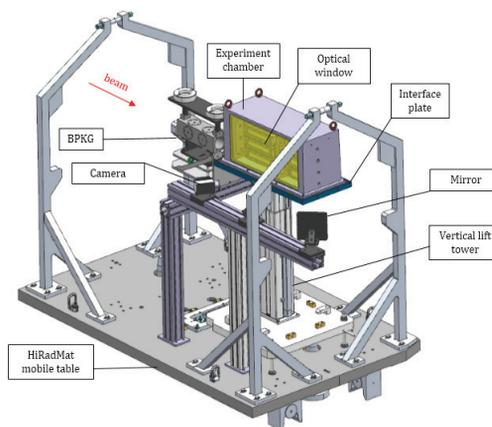
Figure 1: Test chamber positioned on mobile table.
