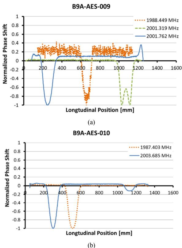
Figure 6: Measured normalized phase shift of the 5<sup>th</sup> pass-band modes in (a) B9A-AES-009 and (b) B9A-AES-010.
