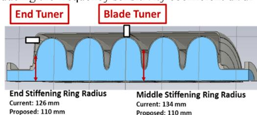
Figure 1: Geometry of the 650 MHz  $\beta=0.9$  5-cell cavity.
