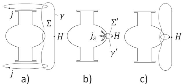
Figure 3: Schematics of the external magnetic field trapped at the quench spot when: a) sustained by the Helmholtz coils current  $\mathbf{j}$  if  $H_{ext} \neq 0$ , b) ideal case when  $H_{ext} = 0$  and c) real case when  $H_{ext} = 0$ .
