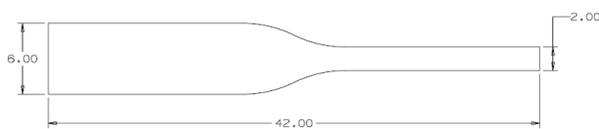
Figure 2: Geometry of the flat fatigue sample, dimensions in mm.
