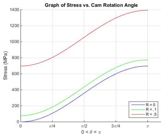
Figure 6: Stress as a function of cam angle for various R-ratios when only varying sample height.
