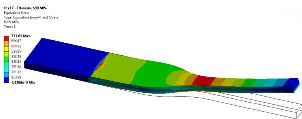
Figure 3: Von-Mises stress results from ANSYS for a flat fatigue sample.
