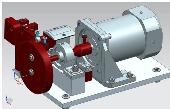
Figure 5: Isometric view of the fatigue testing machine design.
