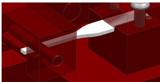
Figure 7: Zoom of sample loaded into the machine with some components shown transparent for clarity.
