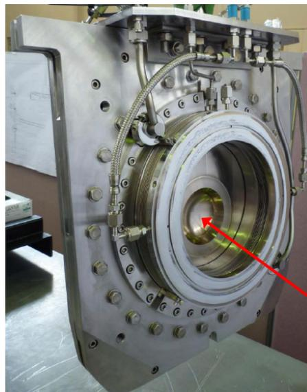
Figure 1: T2K vacuum window assembly, with a red arrow highlighting the approximately 15 cm diameter Ti window.
