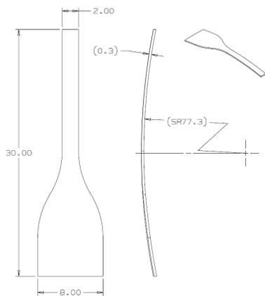
Figure 4: Spherical sample geometry, dimensions in mm.
