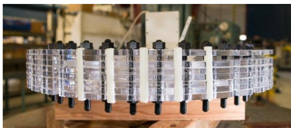
Figure 4: Detail of key and axial rod configuration.
