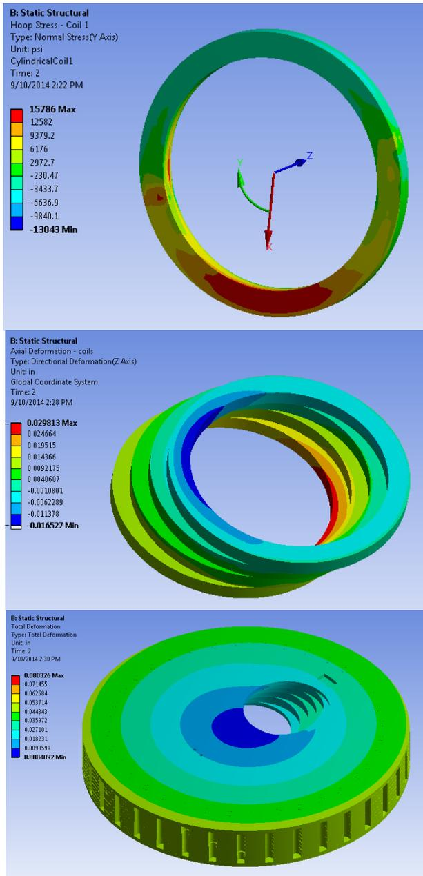
Figure 2: Coil Hoop stress while energized (top). Coil deformation while energized (middle). Coil and structure deformation on cool-down and energization (bottom).
