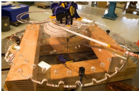
Figure 3: Winding of layer 1.
