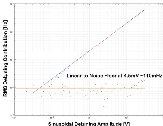
Figure 8: Fast tuner resolution measurements. Piezo driving amplitude vs Noise floor – 5 Hz
