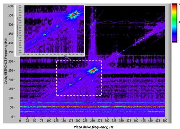
Figure 9: Piezo-to-RF transfer function of the cavity/vessel/tuner system.
