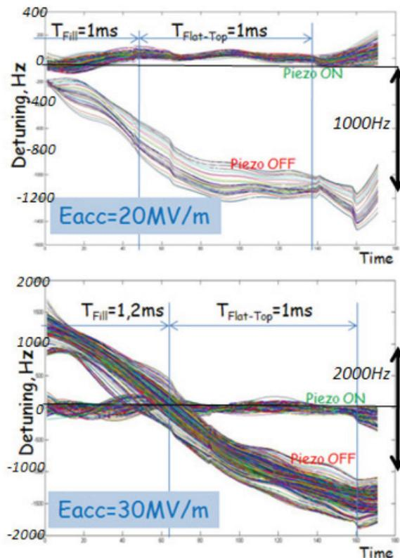
Figure 1: Pulsed compensation of Lorentz force detuning in an SSR1 cavity by adaptive algorithm.
