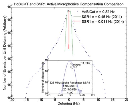
Figure 4: A comparison detuning distributions following active compensation at HoBiCaT and FNAL.
