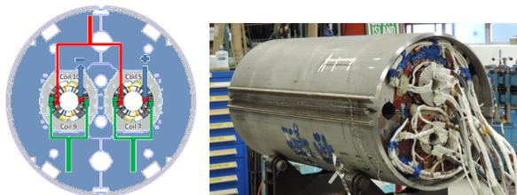
Figure 1: The coil electrical connection (left) and the assembled MBHDP01 cold mass before end plate welding and coil splicing (right).
