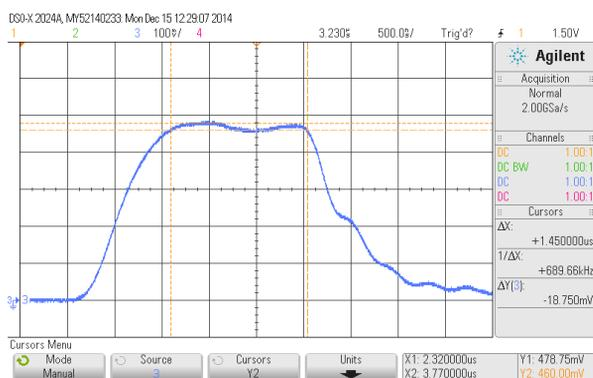
Figure 2: Output pulse voltage with 48 plates, showing 500 kV with staggered plate switching to optimize flat top. 106.2 kV/div, 500 ns/div.
