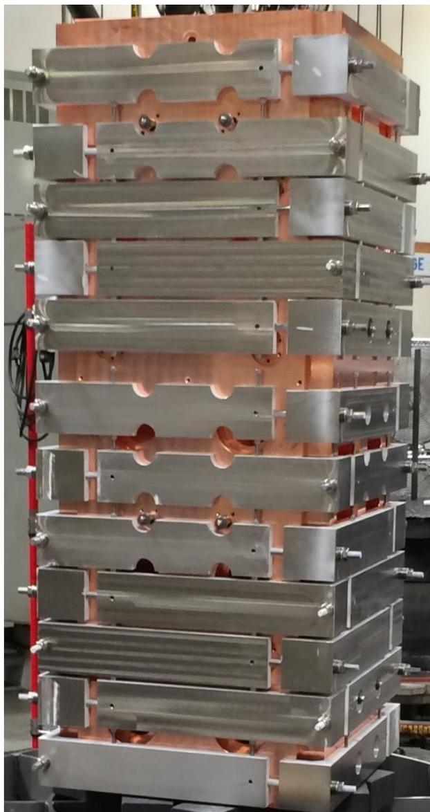
Figure 6: RFQ module with braze fixtures.
