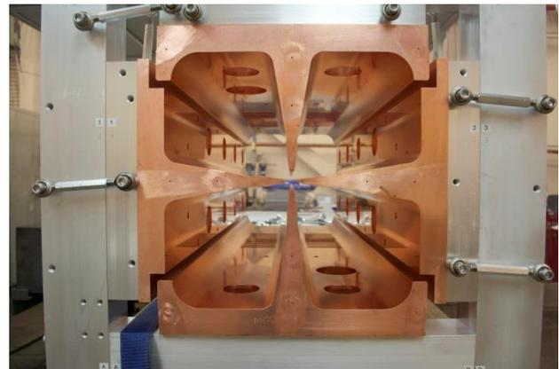
Figure 5: RFQ module in assembly fixture.
