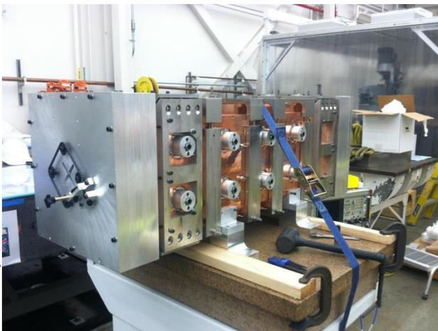
Figure 4: LBNL module 2 prep for bead pull.
