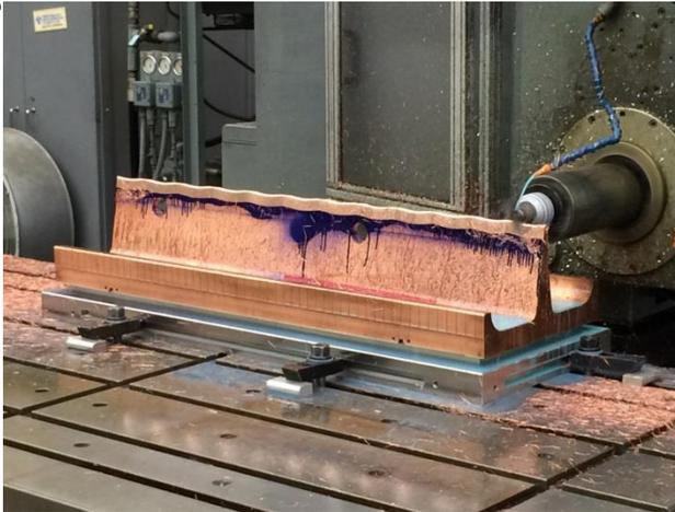
Figure 3: Vane modulations being cut at LBNL
