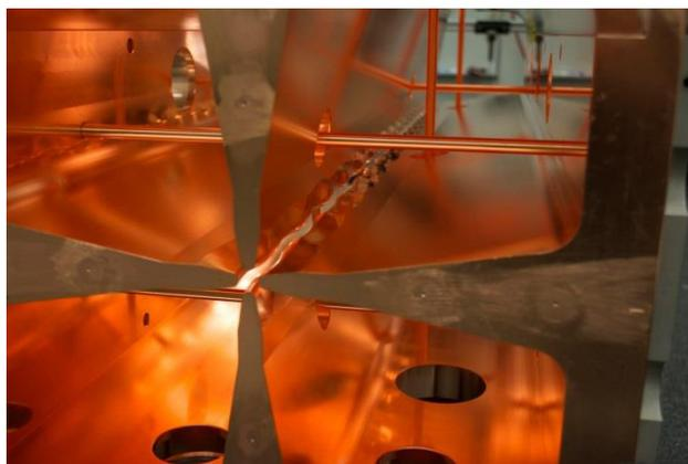
Figure 7: Brazed RFQ inner cavity
