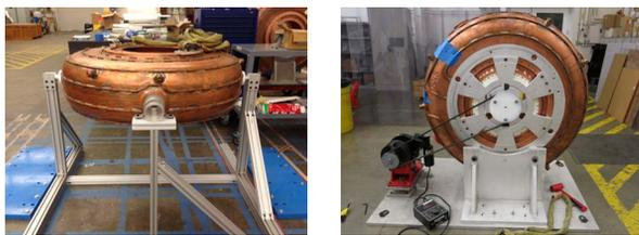
Figure 2: Cavity on the fixture before EP. Left: Rotation fixture from Fermilab; Right: EP fixture.
