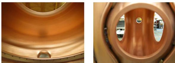
Figure 3: Cavity inner surface after EP.
