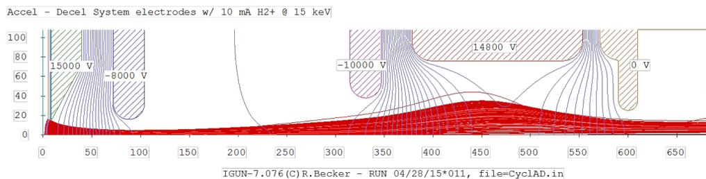
Figure 4: IGUN simulation of beam extraction and matching to RFQ.
