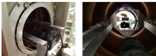
Figure 4: Cavity inspection fixture mounted on the vessel cover plate with the camera outside the vessel (left) and the mirror inside the cavity (right).
