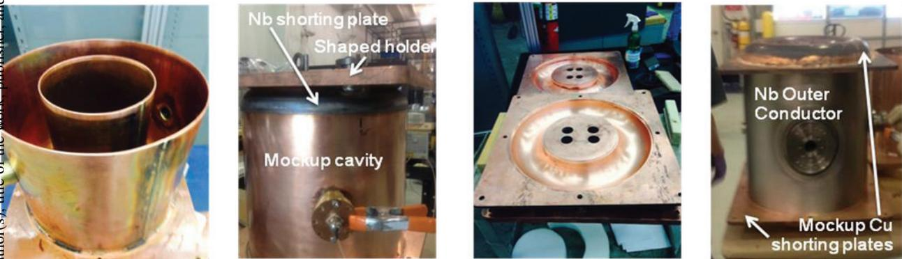
Figure 3: Mock-up cavities and stack up assemblies for FRIB HWRs coarse tuning.
