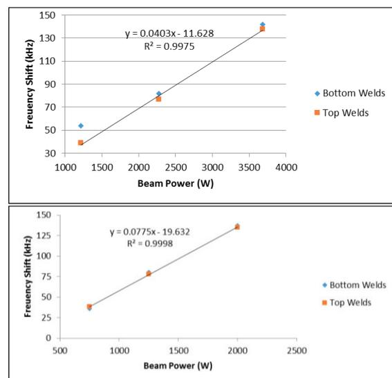
Figure 2. Frequency vs. EB power plot.
