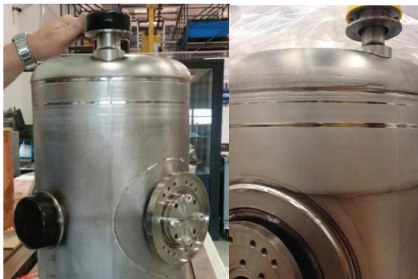
Figure 1: Virtual Welding rings in FRIB  $\beta=0.29$  (left) and  $\beta=0.53$  HWR prototypes, before He vessel installation.
