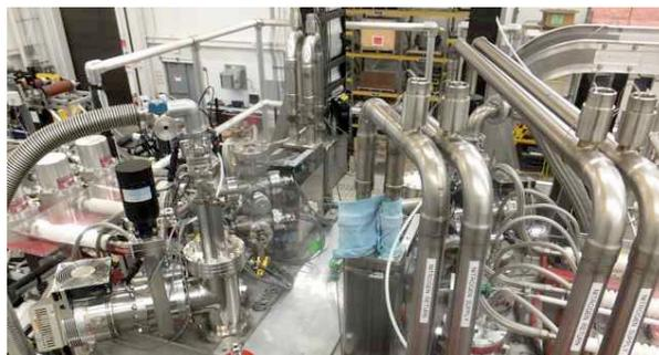
Figure 4: The 4 K cryogenic system for the two cryostats.
