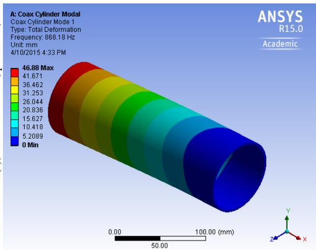
Figure 5: Deformation of the coaxial cylinder at the 868.18 Hz mode .
