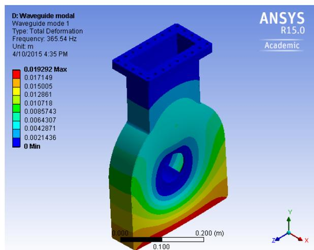
Figure 4: Deformation of the waveguide at the 365.54 Hz mode .
