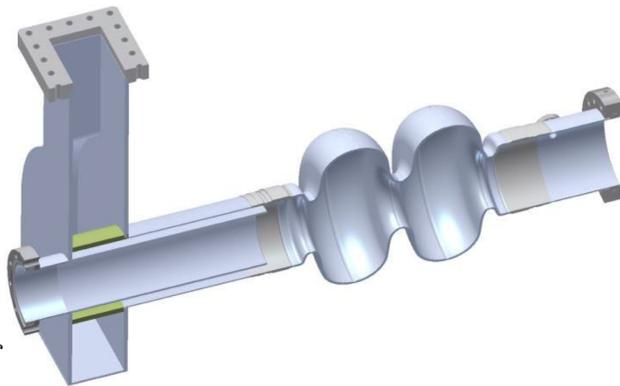
Figure 1: Cornell ERL injector cavity with symmetric coupler taken from [1]
