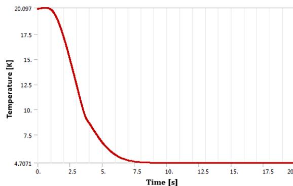
Figure 3: Maximum temperature along the coaxial cylinder over time for initial temperature = 20 K .
