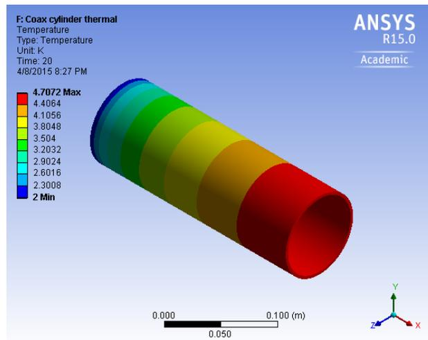
Figure 2: Coaxial cylinder steady state temperature distribution .
