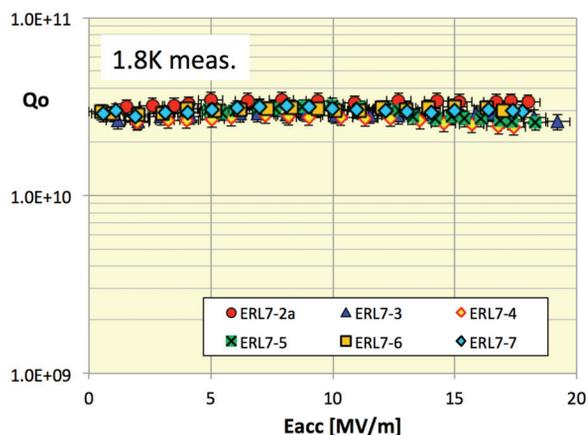
Figure 2: Vertical test results for all 6 ERL cavities. All cavities exceeded the design specifications for the ERL ( $Q=2 \cdot 10^{10}$  at 1.8 K). The reproducibility of the results, gained without any reprocessing of a cavity, is remarkable. The cavities were not N-doped!
