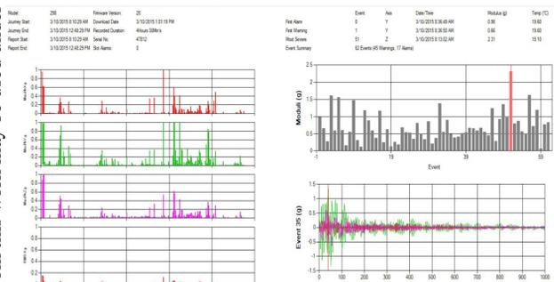
Figure 8: Accelerometer data taken during the transportation of the cryo-module.
