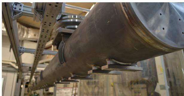
Figure 4: Assembly frame, supporting the HGRP which acts as a strongback for all beam line components, hung under the precision machined mounting feet.
