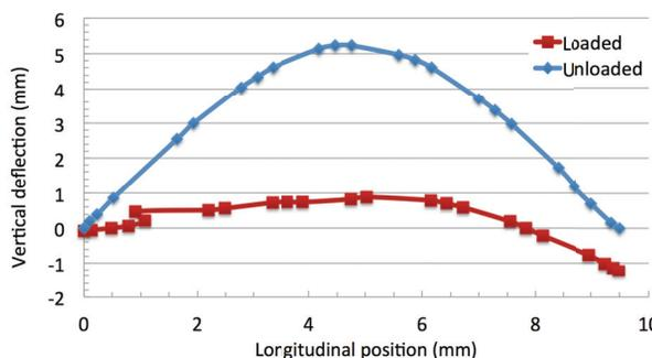
Figure 5: Vertical position of the reference surfaces on the helium gas return pipe defining the positions of all beam line components. In a module string, the right end will receive more support resulting in a better vertical positioning.
