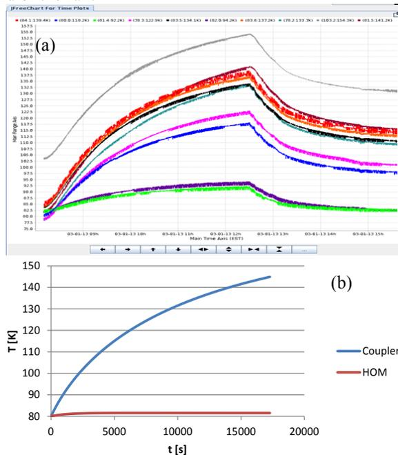
Figure 4: Measured heating of the ICM during a high current run (a) and the simulation results (b).
