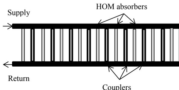
Figure 1: The 80 K cryogenic cooling piping: The thermal intercept of the ten coupler and the 12 channels to cool the higher order mode absorbers a fed in parallel.
