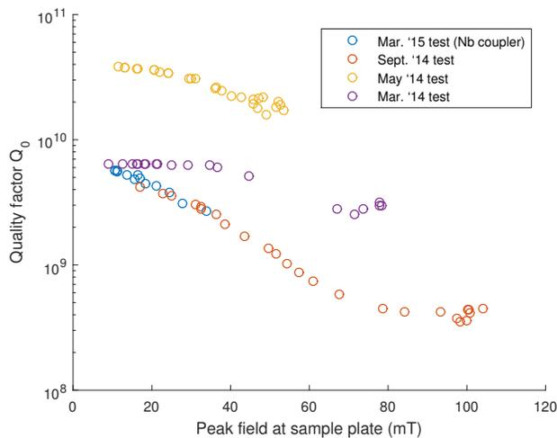
Figure 2: Quality factor  $Q_0$  measured against peak field at the sample plate for several tests. The September 2014 test reached fields of 100 mT, but a significant  $Q$ -slope was observed. The March 2015 test featured a niobium-tipped coupler but did not reach high fields.
