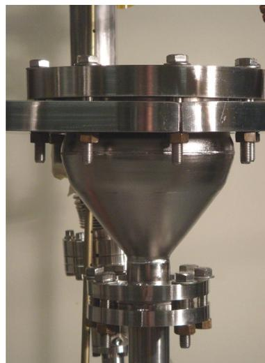
Figure 1: Third-generation Cornell TE sample host cavity.
