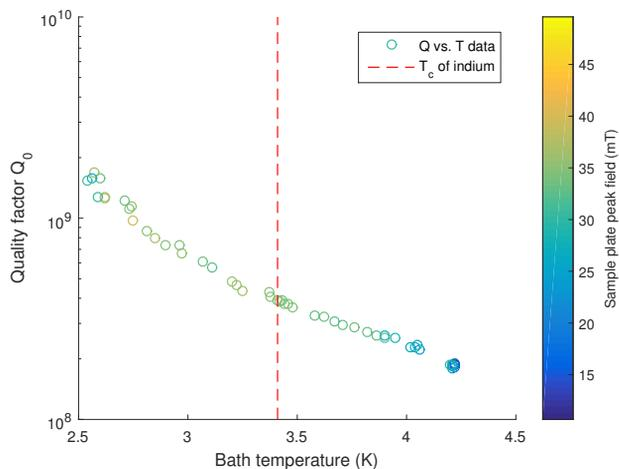
Figure 3: Quality factor  $Q_0$  measured against temperature for the September 2014 test, which exhibited a  $Q$ -slope. Since there is no significant change at the critical temperature of indium, it does not appear that the  $Q$ -slope was caused by indium losses.
