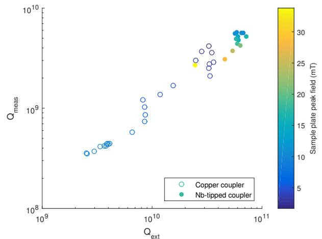
Figure 4: Intrinsic quality factor  $Q_m$  plotted against external quality factor  $Q_{ext}$  for the test with niobium-tipped coupler and a representative copper coupler test. The niobium tip does not appear to decrease the impact of the coupler on the measured quality factor.
