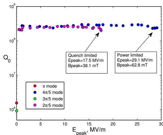
Figure 4: Cavity quality factor for different modes as a function of peak surface electric field at 4K. The drive probe was adjusted to provide near critical coupling to the modes  $2\pi/5$  and  $4\pi/5$ , or max achievable coupling for modes  $\pi$  and  $3\pi/5$ .
