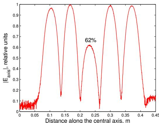
Figure 2: Gradient profile of the tuned cavity obtained from bead-pull measurements. The field in the center cell is intentionally lowered to ensure equal surface magnetic field in every cell.
