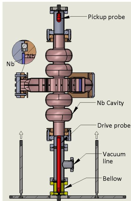
Figure 3: Cross section of the 5-cell module with the pickup assembly and the drive assembly.
