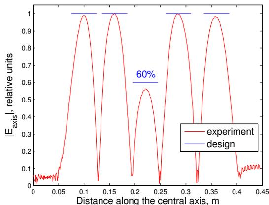
Figure 3: Gradient profile of the tuned cavity obtained from bead-pull measurements.
