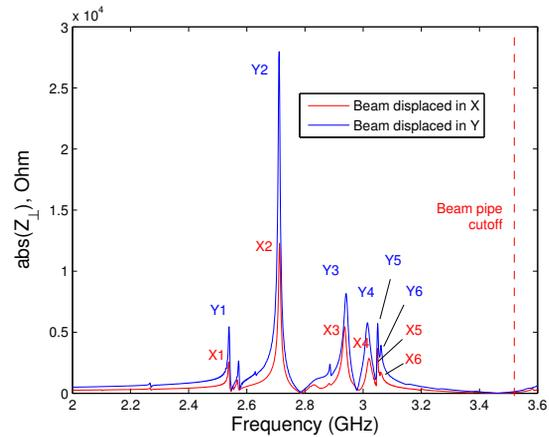
Figure 2: Transverse impedance calculated by CST Particle Studio. 12 most dangerous modes correspond to the biggest peaks in impedance.
