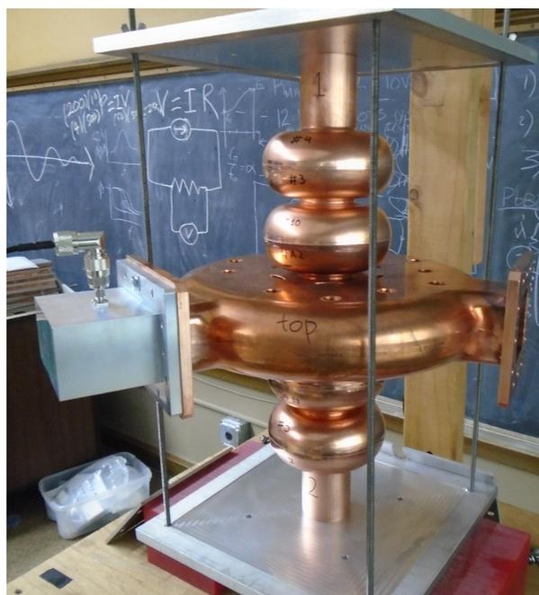
Figure 1: Copper prototype of the 5-cell accelerating module.
