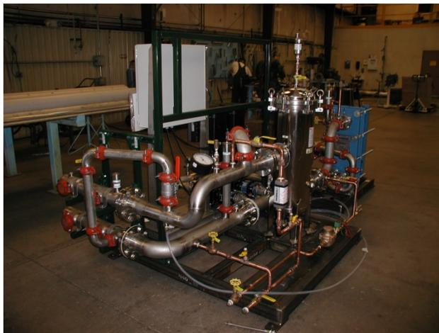
Figure 6: A06 Pump Skid (shown at fabrication facility).
