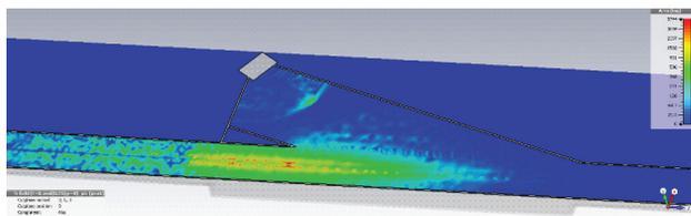
Figure 4: Absolute value of the magnetic field just before the two beams are merged.
