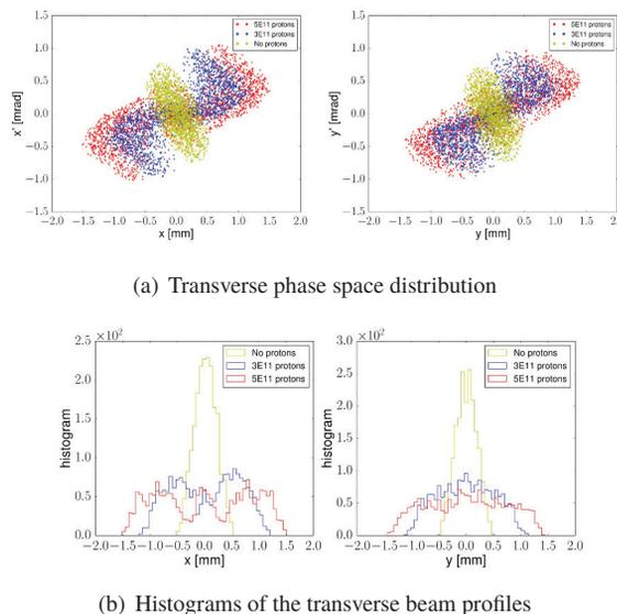
Figure 7: Effect of the beam-beam interaction on the distribution at the entrance of the plasma chamber in case of no,  $3 \cdot 10^{11}$  and  $5 \cdot 10^{11}$  protons.
