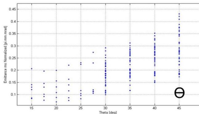
Figure 3: Result of the parametric study of the extraction system to minimize the produced beam emittance.
